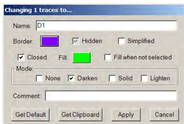
Figure 8.9. The Trace Attributes dialog. The title bar indicates how many traces were selected when the dialog was invoked. All of these traces will receive the changes made in the dialog. Grayed checkboxes or buttons (e.g. the Hidden checkbox) indicate a don't care condition. As long as these boxes are not modified these parameters will not be changed on any of the selected traces.
