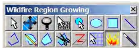
Figure 1.2. The Tools window. This window should be visible at the top of the RECONSTRUCT™ main window. Use the left mouse button to select a tool. The Line Tool used for calibration lines is the 8th button on the top row. The Pencil Tool is the 10th button. The Wildfire tool button is depressed and so a description of the tool appears in the title bar.
