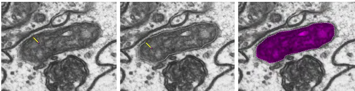
Figure 1.4. Drawing a trace with the freehand drawing tool. (left) Start of the tracing. The pencil is positioned at the profile to be traced and the left mouse button pressed and held down. (middle) Just before release of the mouse button. The pencil left a trail where it was moved with the mouse from the start position. (right) Right after release of the mouse button. The trace is closed and filled with color.
