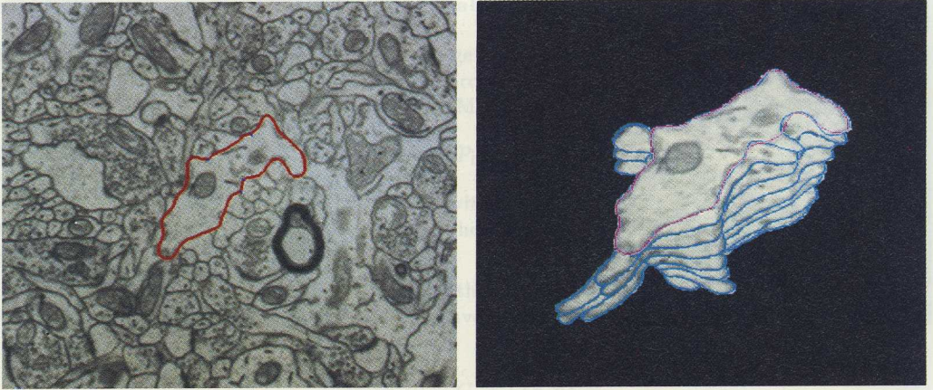
Fig. 4: To the left, the current EM image with a deformable contour (snake); to the right, a stack of dendritic profiles and their interiors. The current snake is displayed in red.
